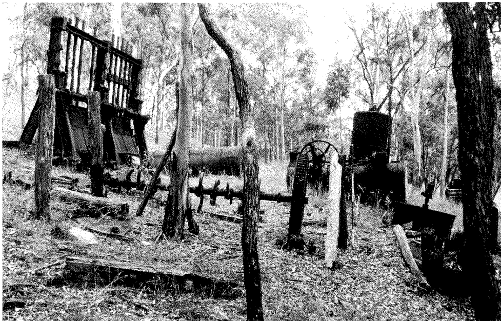
Fig. 4: The United Rise Battery at Monal, near Monto in southern Queensland, retains its stamper battery (to the left), several boilers including a Cornish boiler in its original bed, a portable engine, a small cyanide works, and Wheeler grinding pans (to the right). It has many of the characteristics typical of small-scale gold batteries of the late nineteenth century, to a degree relatively unusual in the state (Criterion D).
